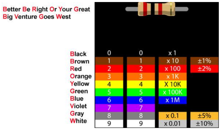
Figure 10.17: Reading the Resistor Color Code. Courtesy of Backward Workshop (William Hunt and Joel Phillips) / CC BY-NC-ND 3.0
