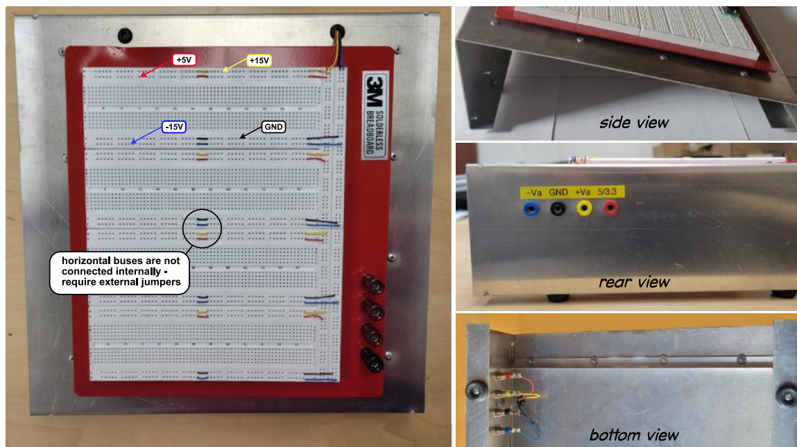
Figure 10.2: Simple breadboard assembly used for analog labs.
