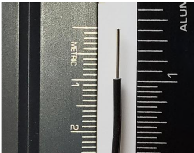
Figure 10.7: A properly stripped jumper wire.
