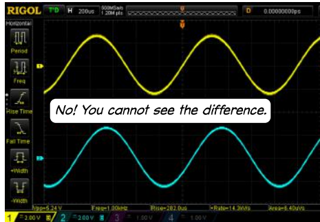
Figure 10.26: It may be difficult to determine the time relationship of traces stacked vertically.
