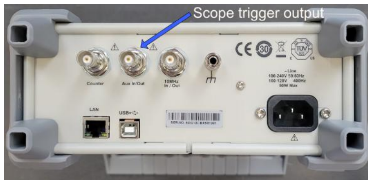
Figure 10.30: Use the function generator trigger output signal to trigger the scope on a sweep waveform.
